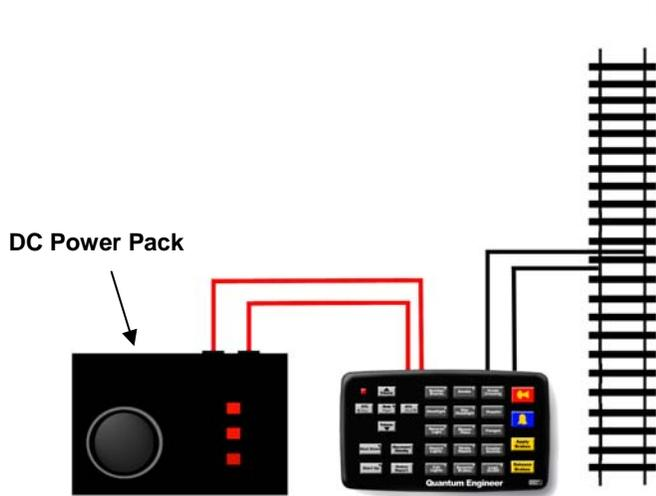
Wiring Quantum Engineer is Simple.
